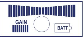
Signal Strength and Polarity (-) or (+) is indicated by the two opposite-facing bar graphs. The signal indications start in the center-most short bars and fill outwardly in increasingly larger bars as the signal increases, until maximum strength is reached.
